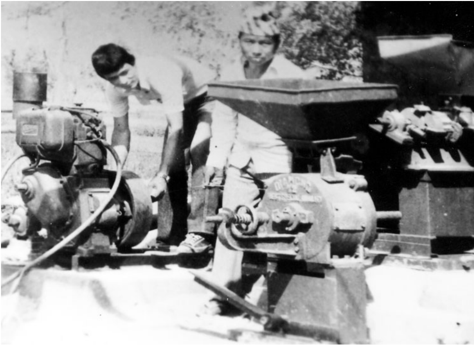
Figure 1 A biogas-powered grain mill with a dual fuel motor. The photograph dates to the early 1980s. Photograph from the Gobar Gas Tatha Agricultural Equipment Development Company archives, courtesy of Mr. Surya Hada.
